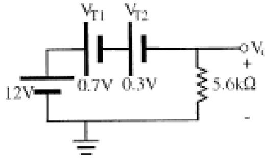
$$E - V_{T1} - V_{T2} - V_0 = 0$$
